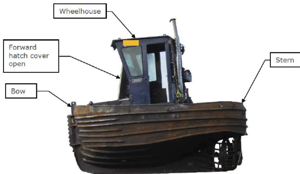
Figure 1: The boom boat, showing the wheelhouse and the forward engine hatch cover fully open. (For more information, see section 2.1 of this report.)
